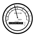
Figure 50. Engine Tachometer
